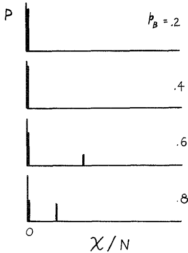
Fig. 2. Probability distributions p of mean failure rate \chi/N for various values of p_B , in unbiased trials with p_A = 1 .
